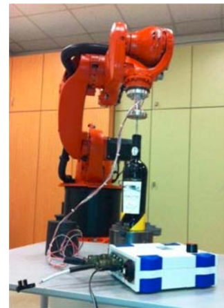
Figure 1 Force measurement by KUKA robot
